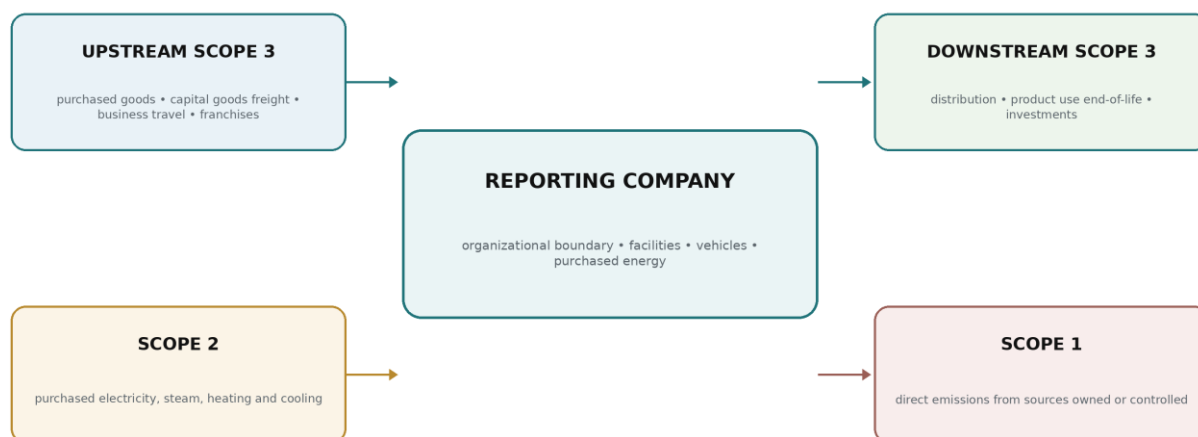
Figure 21.5. Greenhouse-gas inventory boundaries across Scope 1, Scope 2 and Scope 3.
